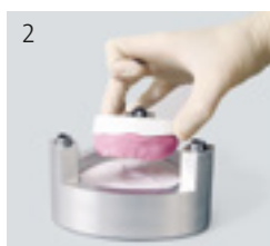
2 Invest the wax-up with the side of the silicone index.
