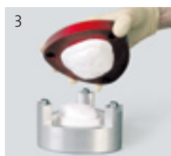
3 Apply plaster to the model and the POLYMASTER lid and close it.
