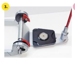
The base plate will be fixed in the upper part of the Candulor plate magnetically, supported by the metal glue. Allow the adhesive to cure for at least 90 min. Only then glue the lower plate.
