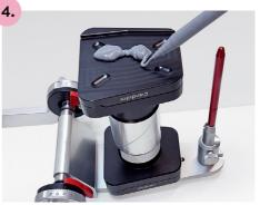
Invert the centring key together with the calibration base plate in the articulator and apply metal glue to the center of the plate.
