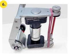
Fix the articulator in place using a rubber band and let the adhesive cure for approx. 90 min.
