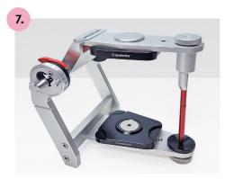
Calibrated CA 3.0 LARGE articulator inclusive plate set for Splitex  $^{\oplus}$  with a height of 126 mm.
