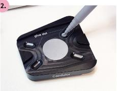
Fill metal glue in the recesses of the base plate marked with "glue dot" and open the articulator, turning it upside-down.
