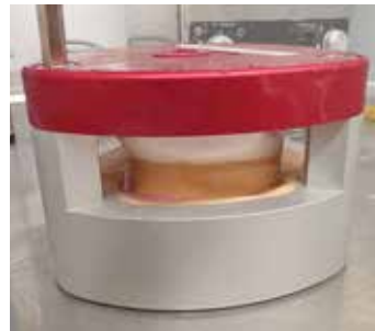
Fig. 17: Models placed in the PolyMaster (cold press)
