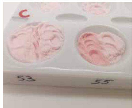
Figs. 21a and b: Individualization of the red esthetics using various resins from the Candulor range. Mixing the polymers 53, 55 and intensive stain powder (ratio 1:1) with the base material 34
