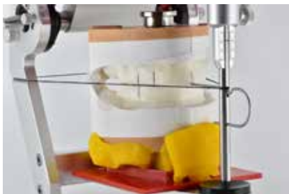
Fig. 7: Alignment of the models to the Camper's plane, visualized with a rubber band.
